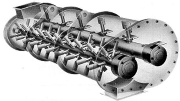
Figure 2. Double-shaft preconditioner.
