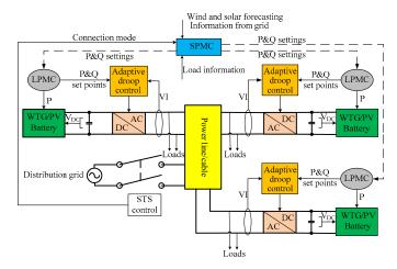
Fig. 4. A roadway microgrid with three EPRTL units and power management system.
