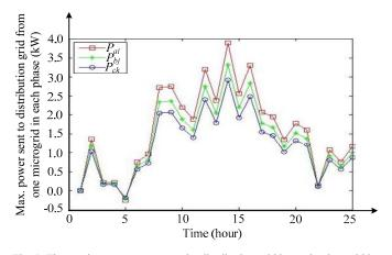
Fig. 5. The maximum power sent to the distribution grid by each microgrid in Phases A, B and C in each hour of a day.
