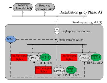
Fig. 1. Typical configuration of a single-phase roadway microgrid.
