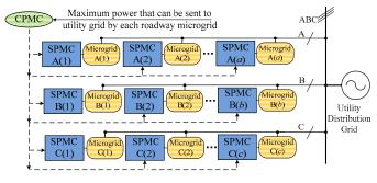
Fig. 2. The architecture of multiple single-phase roadway microgrids integrated into a three-phase distribution grid.
