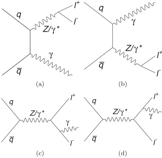
FIG. 1. Feynman diagrams for leading-order  $Z\gamma$  production in the SM: (a) and (b) initial-state radiation from one of the initial-state partons; (c) and (d) final-state radiation from one of the final-state leptons.
