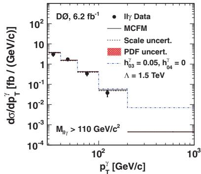
FIG. 5 (color). The SM prediction and anomalous  $Z\gamma$  coupling production compared with the unfolded  $d\sigma/dp_T^\gamma$  for combined muon and electron channels for  $p_T^\gamma > 30 \text{ GeV}/c$  and  $M_{\ell\ell\gamma} > 110 \text{ GeV}/c^2$ .
