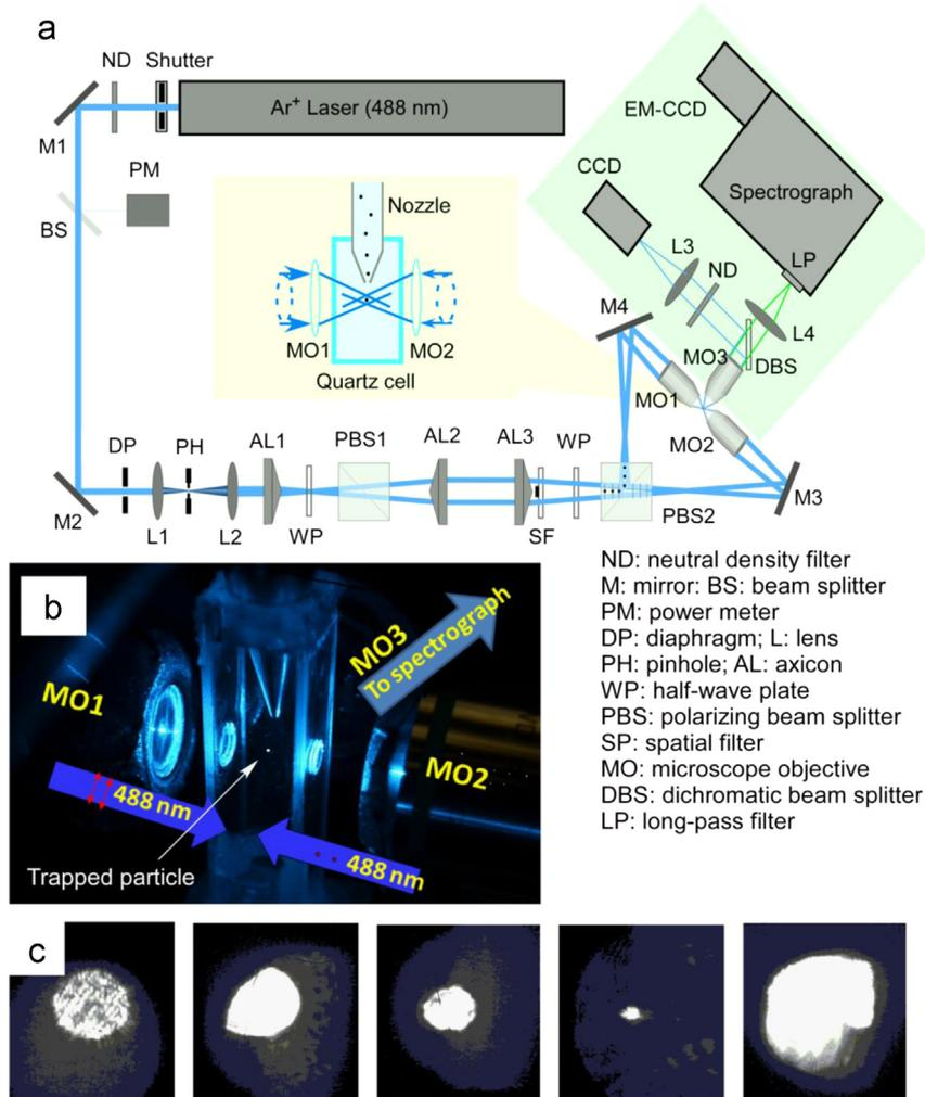
**Fig. 1.** Schematic of the photophoretic trapping-Raman spectroscopy (PTRS) system: (a) optical arrangements; (b) an image of the key trapping components and the location of the trapped particle; and (c) images of trapped particles, from the left to the right: single wall carbon nanotubes (SWCNT), English oak, ragweed, ryegrass, and Bermuda grass smut spores.
