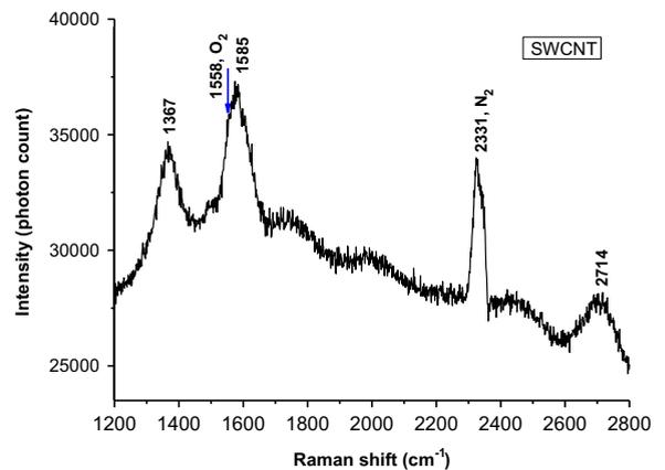
**Fig. 3.** Photophoretic trapping Raman spectra of a single particle ensemble of graphitized single wall carbon nanotubes (SWCNT) trapped in air in the closed quartz cell.
