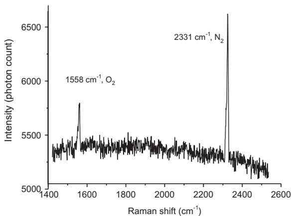
**Fig. 2.** Raman spectra of ambient  $O_2$  and  $N_2$  recorded for wavenumber calibration of the photophoretic trapping Raman spectroscopy system. The excitation wavelength was 488 nm. The entrance slit width of the spectrograph was 50  $\mu\text{m}$ .
