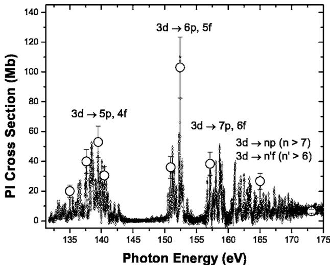
FIG. 5. Photoionization cross section in the energy range of  $3d \rightarrow np$  ( $n > 4$ ) and  $3d \rightarrow nf$  ( $n > 3$ ) transitions in  $\text{Kr}^{5+}$  measured with an energy resolution of 100 meV. The large open circles with error bars represent the absolute cross-section measurements and their uncertainties.
