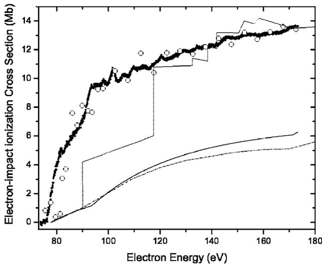
FIG. 6. Energy-scan measurement of the cross section for electron-impact ionization of  $\text{Kr}^{5+}$  (filled circles) normalized to the absolute measurement of Bannister *et al.* [10] (open circles). The experimental energy resolution is approximately 1 eV. The solid curve is the Lotz formula prediction for the direct ionization cross section. The dot-dashed and dotted curves are direct and total ionization cross sections calculated by Gorczyca *et al.* [14], respectively.
