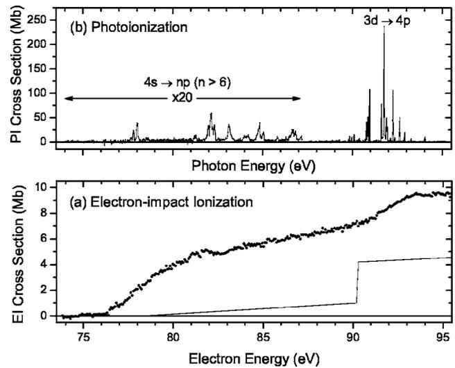
FIG. 7. Comparison of electron-impact ionization cross-section measurements for  $\text{Kr}^{5+}$  (a) with photoionization cross-section measurements (b) in the energy range 73.8 to 95.5 eV. The photoionization cross section in the energy region from 74 to 87.2 eV has been multiplied by a factor of 20. In (a), the curve is the theoretical ionization cross-section calculation from Ref. [14].
