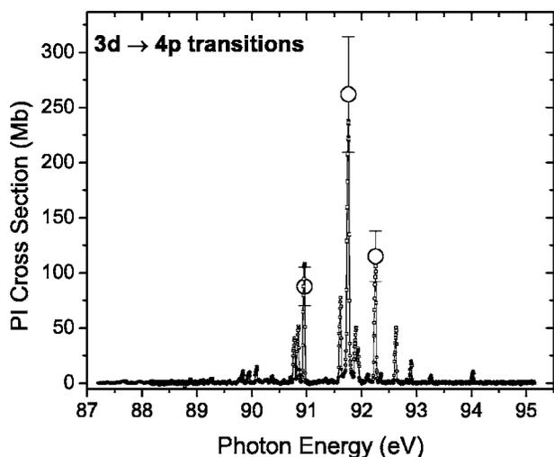
FIG. 3. Absolute photoionization cross section for the  $3d \rightarrow 4p$  transition in  $\text{Kr}^{5+}$  measured with an energy resolution of 50 meV. The large open circles with error bars show absolute cross-section measurements made at the same energy resolution, with their estimated uncertainties.
