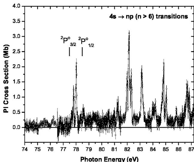
FIG. 1. Absolute photoionization cross section of  $\text{Kr}^{5+}$  measured with a photon energy resolution of 100 meV, showing  $4s \rightarrow np$  transitions. The vertical bars indicate the ionization thresholds for the  ${}^2P^0_{3/2}$  metastable state and the  ${}^2P^0_{1/2}$  ground state.
