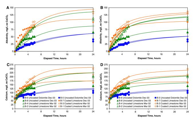
**Fig. 1** Concentrations of alkalinity and calcium as CaCO<sub>3</sub> with elapsed time of contact between Bell Discharge effluent and uncoated or Fe(OH)<sub>3</sub>-coated calcitic limestone or uncoated dolomitic limestone in collapsible, closed-containers (cubitainers): **a** Alkalinity, first-order curve; **b** alkalinity, second-order curve; **c** Ca, first- order curve; **d** Ca, second-order curve. Calcitic limestone immersed in flowing effluent
