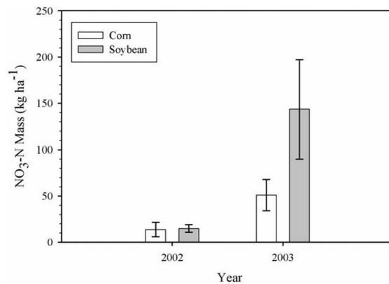
**Figure 4.** Masses losses of  $\text{NO}_3^-$ -N in leachate from lysimeters in 2002 and 2003 as related to the previous year crop (2001, corn or soybean). For each year the mass losses are averaged over the nitrogen treatments for each previous crop. Error bars are the standard error of the treatment means.
