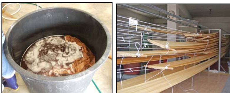
Figure 21. Bleaching procedure-hemp fabrics in the caustic soda solution. Photograph by the author. Figure 22 (right). Drying hemp fabrics on the drying rack. Photograph by the author.
