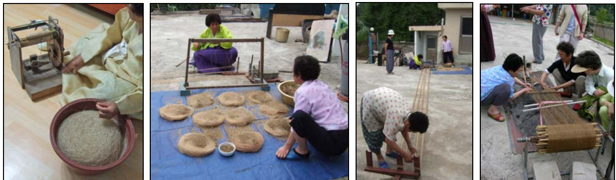
Figure 14(left). Winding an oblong bundle of weft yarn using the bobbin winder. Photograph by the author.
