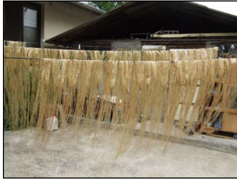
Figure 10. Drying hemp fiber layers. Photograph by the author.
