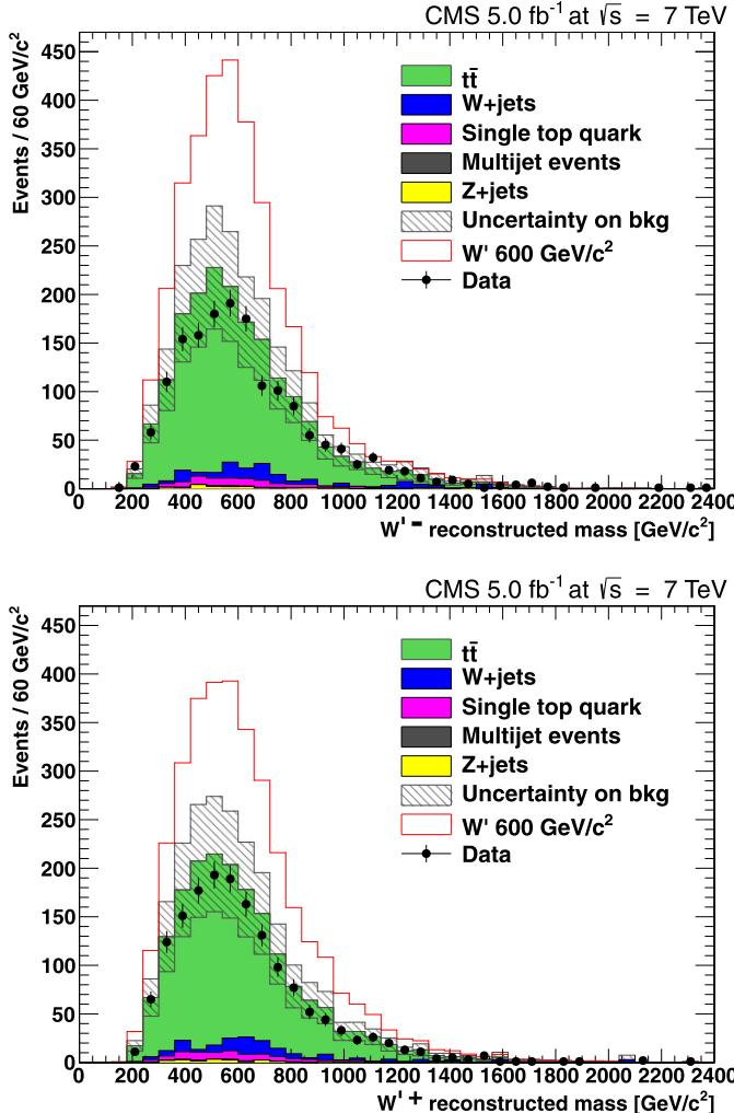
**Fig. 3.** Invariant mass distributions for (top)  $W'$ − candidates and (bottom)  $W'$ + candidates. The figures show a comparison between the background prediction, with candidates reconstructed from simulated signal events stacked on top, and data. Uncertainty bands represent statistical and systematic uncertainties on the background prediction.
