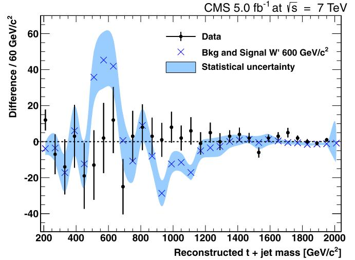
**Fig. 4.** Difference in yields for  $W'$ − and  $W'$ + candidate invariant mass distributions. Data are compared with the combination of background and a simulated  $W'$  signal with a mass of 600  $\text{GeV}/c^2$  and  $g_L = 0$  and  $g_R = 2$ . The shaded blue band indicates the statistical uncertainty of the signal and background combination. (For interpretation of the references to color in this figure legend, the reader is referred to the web version of this Letter.)
