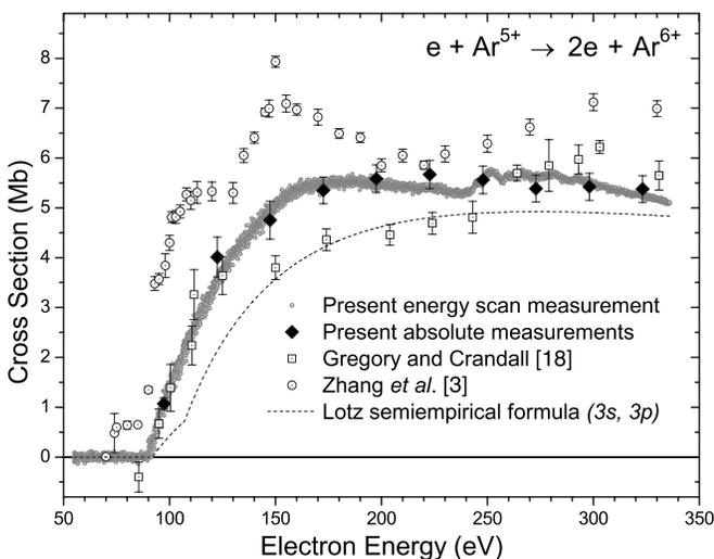
FIG. 5. Comparison of current cross-section measurements for electron-impact ionization of  $\text{Ar}^{5+}$  with previous measurements and with the Lotz semiempirical formula prediction for ionization of the  $3s$  and  $3p$  subshells.
