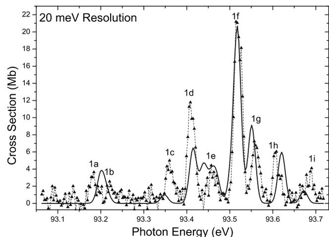
FIG. 4. Comparison between predicted and experimental results for the first resonance in Fig. 3. The dashed curve with triangle symbols is the experimental result, taken at a resolution of 20 meV. The solid curve is a calculation convoluted with a Gaussian profile, 20 meV FWHM, shifted by +1.23 eV.
