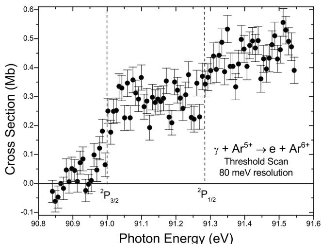
FIG. 1. Photoionization cross-section measurement in the threshold energy region at a spectral resolution of 80 meV. The dashed lines indicate the thresholds of the  ${}^2P_{1/2}$  ground state and the  ${}^2P_{3/2}$  metastable state determined from these measurements.
