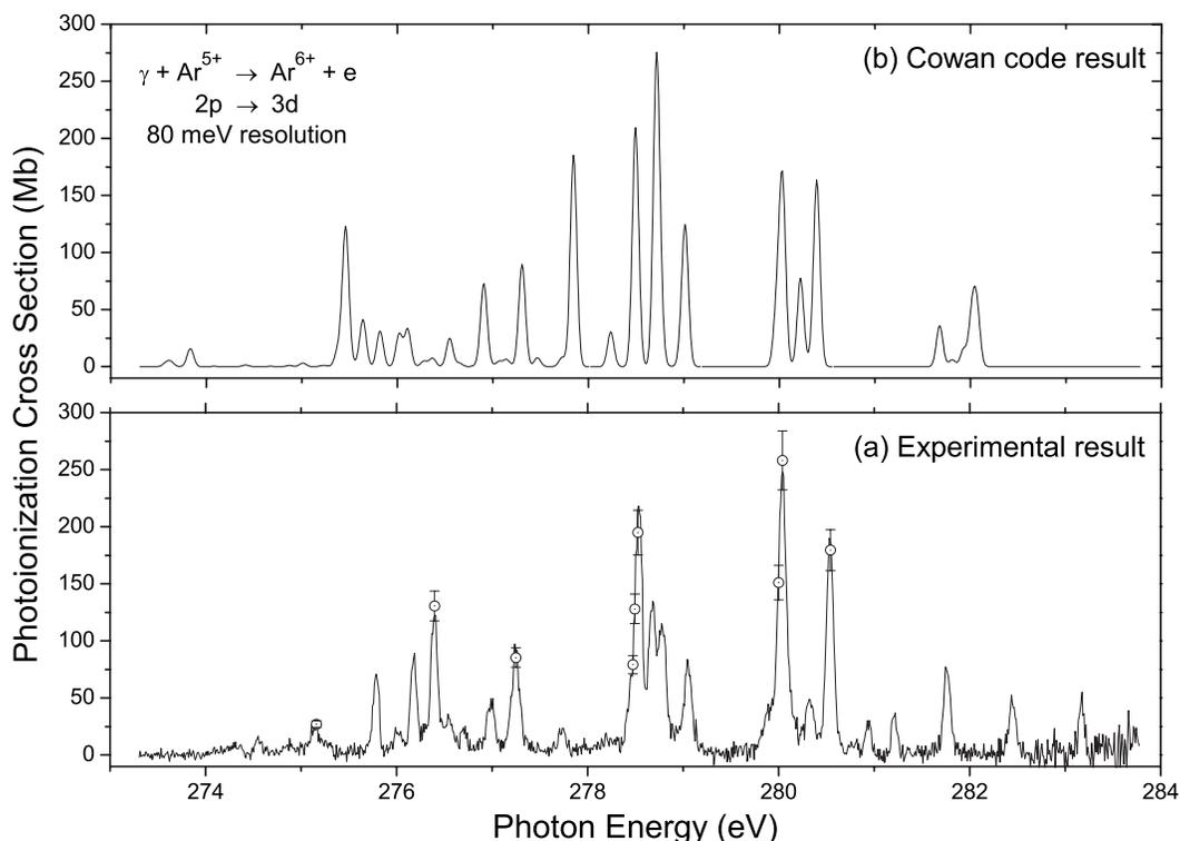
FIG. 2. Comparison of cross-section measurements for photoionization of  $\text{Ar}^{5+}$  in the energy range of 273–284 eV taken at a resolution of 80 meV with a resonance spectrum calculated using the Cowan atomic structure code. The calculation was convoluted with a Gaussian profile of 80 meV FWHM. The open circles with error bars are absolute measurements.
