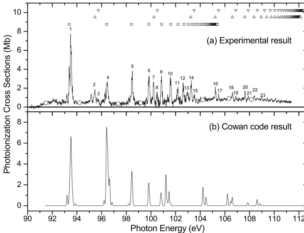
FIG. 3. Comparison of absolute cross-section measurements for photoionization of  $\text{Ar}^{5+}$  with the calculated spectrum in energy range of 90–111 eV. The energy scale of the calculated spectrum has been shifted by +1.23 eV in this case to better match the experiment. Open circles are absolute measurements.
