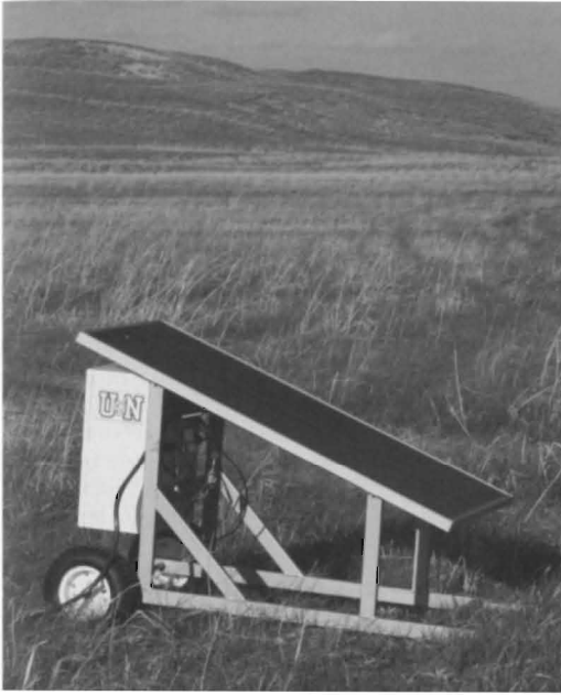
Figure 5.1. The solar power system used to support a digital video recorder, housed in the weatherproof case at left. Cables run 31 m from the power source and recorder to a camera at the nest. The system is shown on our study site during 2006 at the Gudmundsen Sandhills Laboratory in Grant, Hooker, and Cherry counties, Nebraska.
