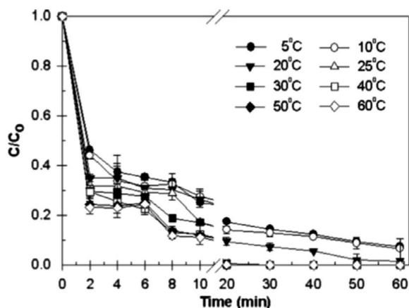
**Figure 6.** Effect of temperature on Pb(II) removal by 0.1 g Z-nZVI from 100 mL of aqueous solution containing 100 mg Pb(II)/L. Error bars indicate standard deviations of the means; where absent, bars fall within symbols.
