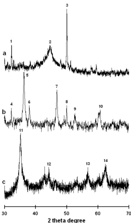
**Figure 7.** XRD patterns of (a) the Z-nZVI; (b) Z-nZVI after shaking with aqueous solution alone; and (c) Z-nZVI after shaking with aqueous solution containing 250 mg Pb(II)/L. 1,4 =  $\text{SiO}_2$ ; 2,12 =  $\text{Fe}^0$ ; 3,8 =  $\gamma\text{-Fe}_2\text{O}_3$ ; 5–10, 13 = iron oxides; 11,14 =  $\text{Pb}^0$ .
