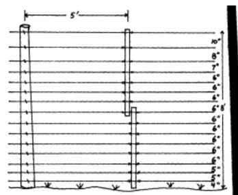
Figure 2--Construction of a portion of a 15 wire high-tensile wire fence showing t) wire spacing. The wood posts are space 25 ft. apart with 4 sets of stays between each set of wood posts.
