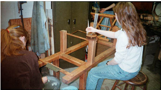
Figure 6 (left). Smith College students Beth Caton and Vanessa Larson reeling silk on their replica of the popular 1830's Piedmont reeler, constructed in the Clark Science Center machine shop for the Northampton Silk Project.
