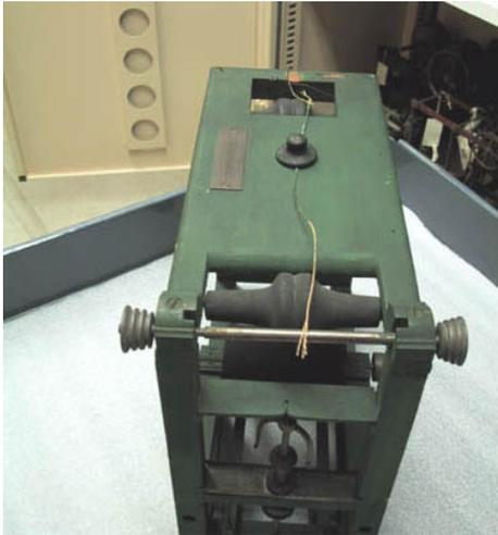
**Figure 8.** Harold Kelsea's patent model, National Museum of American History (Maryland storage facility.) The broken cord represents the "endless band" M to which the knobs N and O are attached (only one can be seen); the hitching knob P was mounted on the bare spot at the far end.
