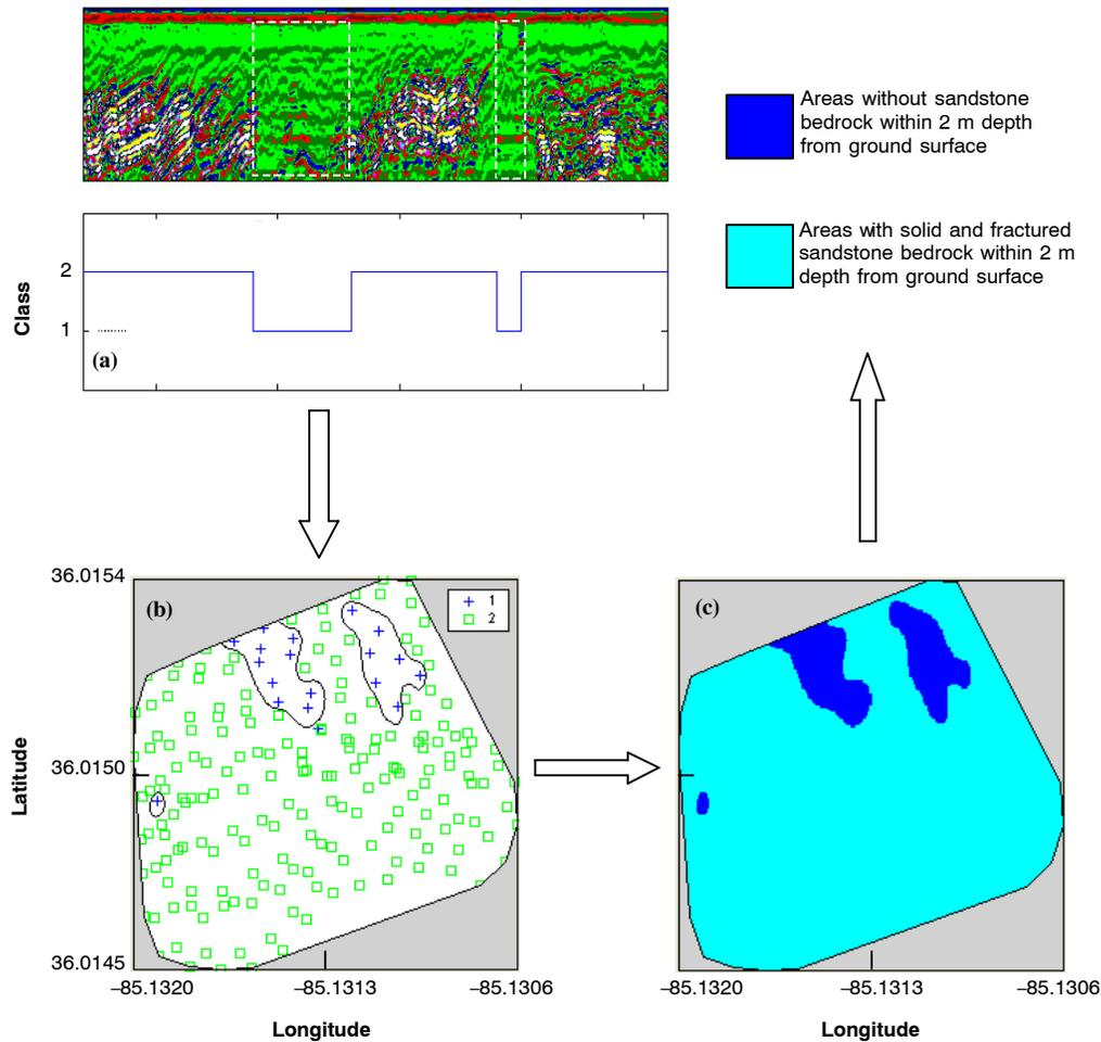
**Figure 4.** (a) How the program separated the subsurface profile into two categories (areas without bedrock and areas with bedrock), (b) how markers on the GPR data were assigned to the different categories and surface plotted, and (c) a surface map showing areas without and with sandstone bedrock.
