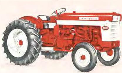
**6-plow International 660.** Choice of 6-cylinder gasoline, direct-start Diesel, or LP-Gas engines. Max. hp 85.21 PTO, 72.81 drawbar on gasoline.
