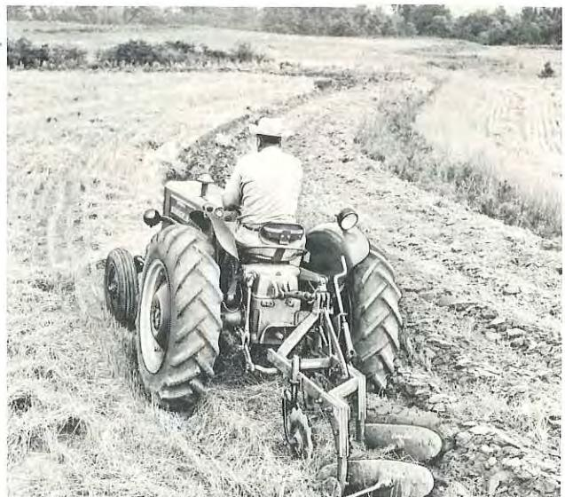
Here's versatility and precision unmatched in the 3-point hitch field. Sway chains allow plenty of flexibility for working contours to perfection. Equipment is leveled with the easy-to-reach hand crank . . . depth is maintained with mechanical precision, and equipment is effortlessly raised and lowered hydraulically. Add it up, there isn't a 2-3-plow Diesel that can hold a candle to the new B-275.
