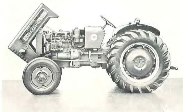
The convenient automotive-type hood feature gives you complete engine access from radiator to fuel tank. Just release the latches, rotate the hood forward and perform routine service with unequalled ease. Minimum maintenance easily accomplished — that's another way you save with a B-275.
