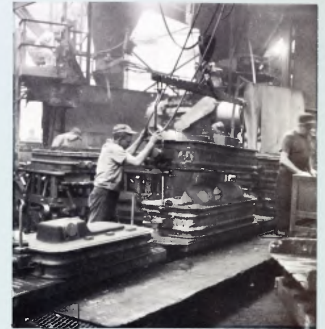
Here a workman prepares a mold for two rear-axle housings. Coming up—the oil pan for a crankcase.
