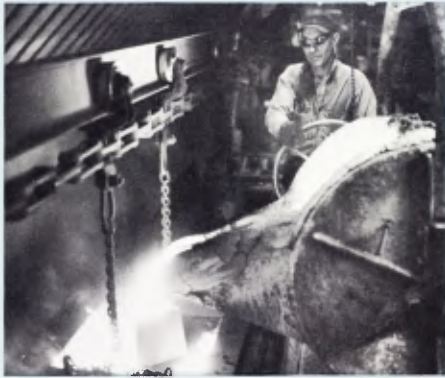
As completed molds move along a conveyor, metal is poured into each one. Besides this method, automatic pouring machines are used.
