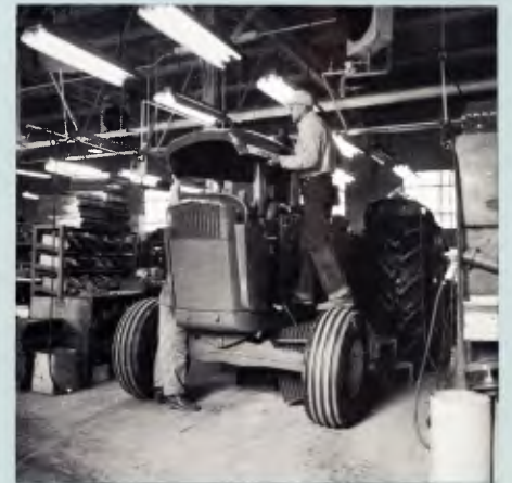
Muffler, hood (above), and side shields are installed on this "5010" Tractor. Hood design permits easy removal for servicing.
