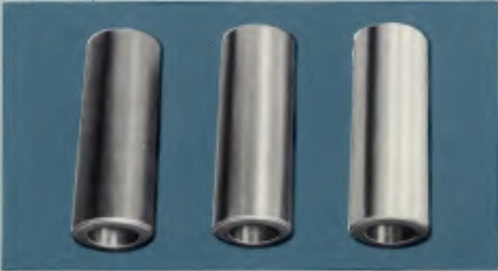
From the cutting machine, a piston pin goes through a ground finish to the mirror-like polish provided by centerless grinders.
