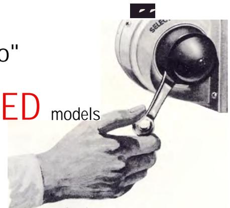
You'll reduce time wasting stops and put more "go" into your farming with Ford's new Select-O-Speed. Yes, a light touch on the Select-O-Speed lever is all you need to shift to any gear—at any time! It's fully selective. And the wide range of overlapping speeds—from as low as .6 mph up to 18 mph—provides outstanding efficiency for any power requirement.
