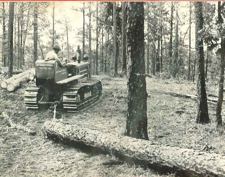
Snaking logs out of the trackless forests supplies work for many TD-6 TracTracTors in logging sections, and with a five-speed transmission, moves more board feet per day.
