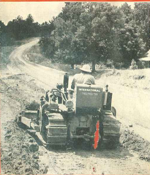
This TD-6 digs and side casts dirt with an 8-foot bullgrader blade.
