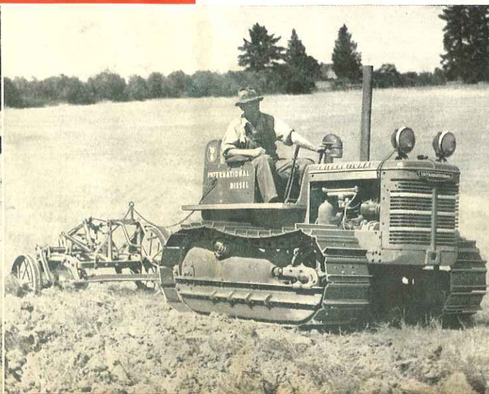
Ample power for pulling three 14-inch plows eight inches deep in northwestern soils.
