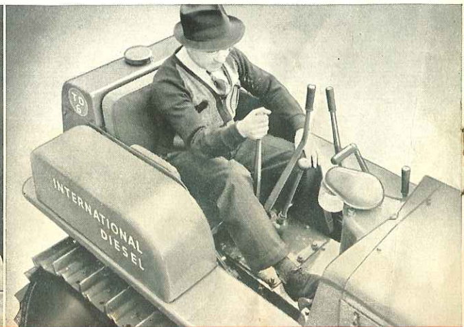
Drivers appreciate the upholstered comfortable seat, adjustable steering levers and brake pedals, convenient controls, unobstructed view ahead and of pulled machines, and the easy, positive-starting engine, which results in increased daily output.
