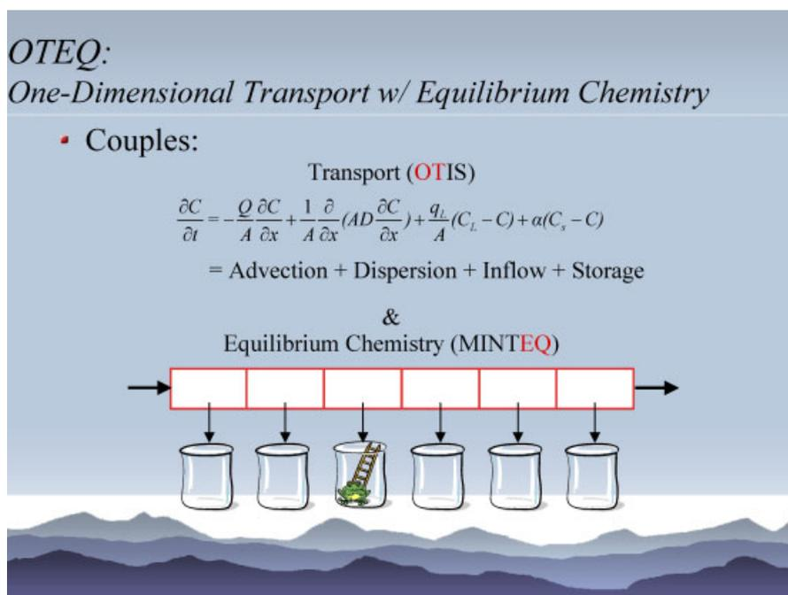
Figure 2. OTEQ combines the stream transport capability of OTIS and the geochemical capability of MINTEQ. Solutes are transported downstream subject to the physical processes of advection, dispersion, inflow and storage. Geochemical calculations within each stream segment quantify sorption and precipitation/dissolution reactions under the assumption of chemical equilibrium
