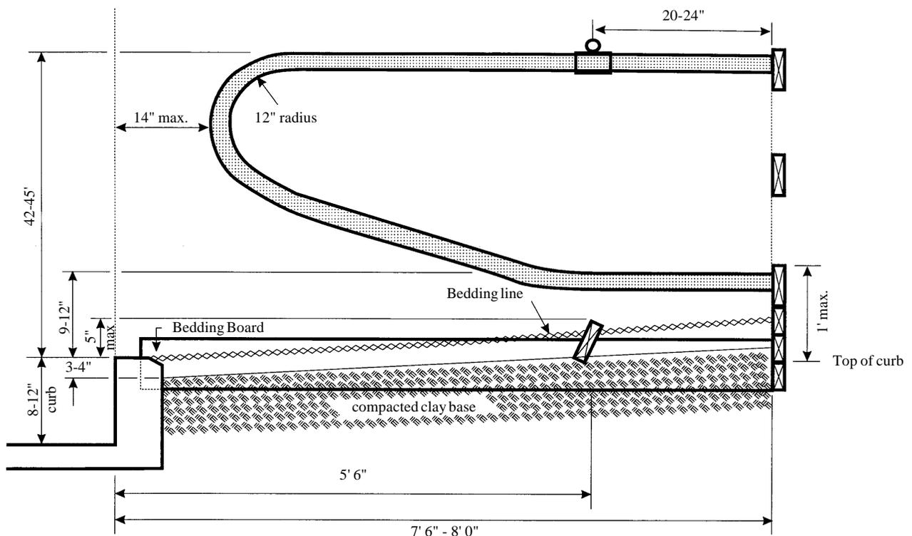
Figure 1. Typical free-stall dimensions.
