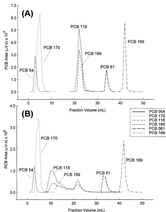
Fig. 1. Summary of GC-ECD analysis of 50 consecutive 1-ml fractions of HPLC eluent from PGC column using the solvent program in Table 1. PCB window mix elution showing mono-*ortho* PCBs, 118 and 189, overloading with each PCB component at 0.1  $\mu\text{g}$  (A), compared to each PCB component at 0.5  $\mu\text{g}$  (B).
