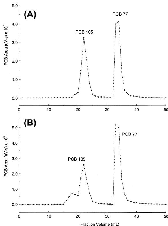
Fig. 4. Summary of GC-ECD analysis of 50 consecutive 1-ml fractions of HPLC eluent from PGC column using the solvent program in Table 1. Effect of non-*ortho* PCB 77 on mono-*ortho* PCB 105. Shows (A) 3  $\mu\text{g}$  PCB 77, 1  $\mu\text{g}$  PCB 105; (B) 5  $\mu\text{g}$  PCB 77, 1  $\mu\text{g}$  PCB 105.
