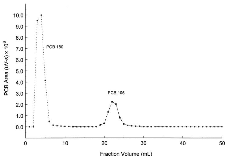
Fig. 3. Summary of GC-ECD analysis of 50 consecutive 1-ml fractions of HPLC eluent from PGC column using the solvent program in Table 1. Shows loading of PCB 180 at 10  $\mu\text{g}$  while monitoring PCB 105 at 1  $\mu\text{g}$ .
