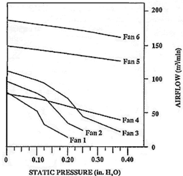
**Figure 2. Performance curves for six 20-inch diameter propeller fans equipped with 1/4 hp motors.**
