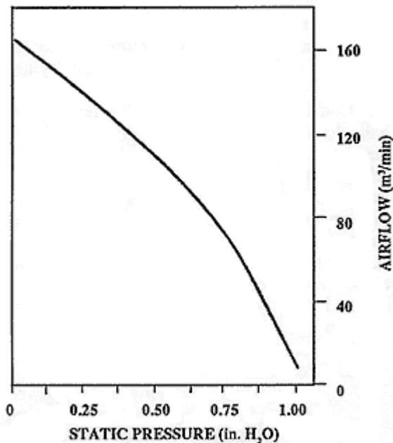
**Figure 1. Fan performance curve (typical, for one fan)**
