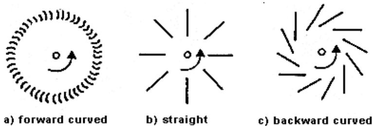
Figure 6. Schematic of centrifugal fan blade configurations.
