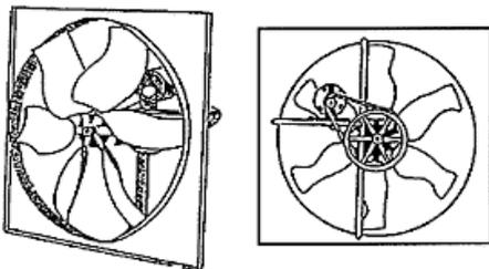
b) Belt-drive fan, front and rear view.
