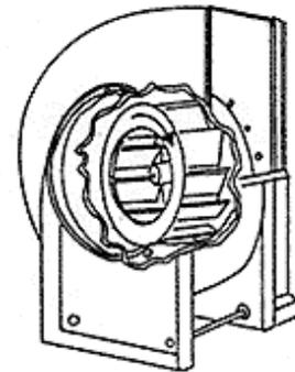
Figure 5. Centrifugal fan.
