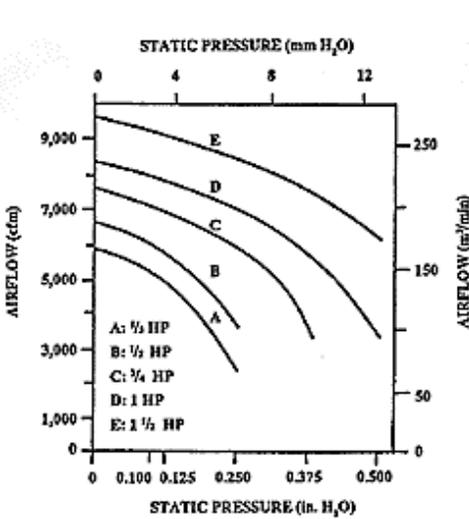
**Figure 7. Performance curves for five ventilation fans from one manufacturer. All fans are 24 inches in diameter and are direct-driven.**
