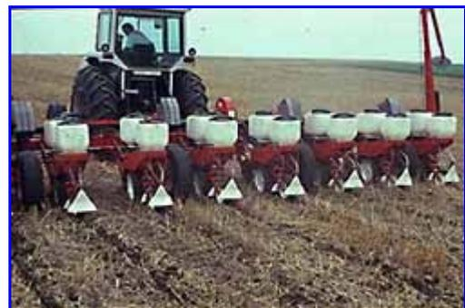
Figure 1. No-till planter working in heavy residue.
