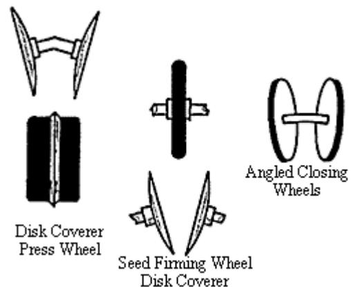
**Figure 5. Types of seed covering and firming devices**
