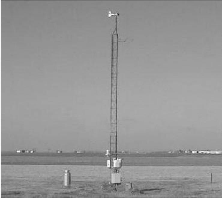
Fig. 1-5. A typical automated weather station, Bondville, IL.
