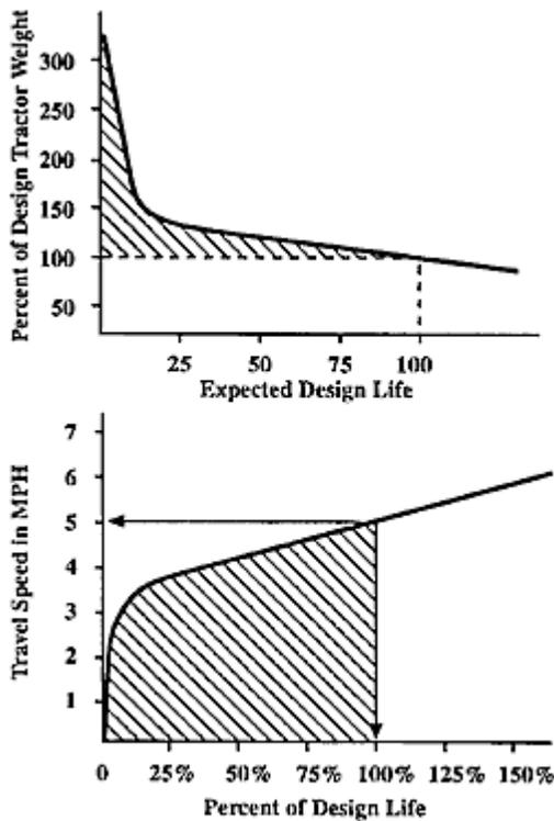
**Figure 2. Design life of final drives is reduced with extra ballast and overfueling the engine (top graph). The reduction is a result of overloading the design requirements of the tractor. The major component that determines the design life of a final drive is the tractor's operating speed (bottom graph). Few final drives are designed to operate at maximum power in the lowest transmission gears.**
