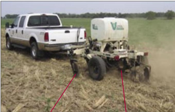
Apparent electrical conductivity mapping unit comprised of six coulters that provide two depths of investigation (0-1 ft and 0-3 ft).
