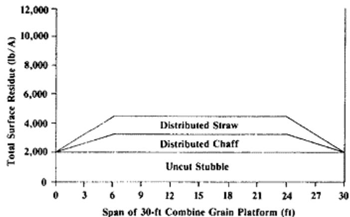
**Figure 4. Near ideal distribution of straw and chaff by a combine equipped with spreader for chaff and straw capable of spreading over a 24- to 30-ft span. Residue left in windrows interferes with herbicide application, tillage, and planting operations.**
