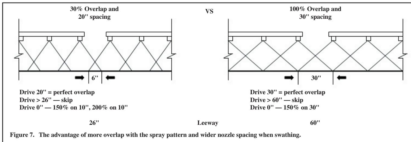
Figure 7. The advantage of more overlap with the spray pattern and wider nozzle spacing when swathing.
