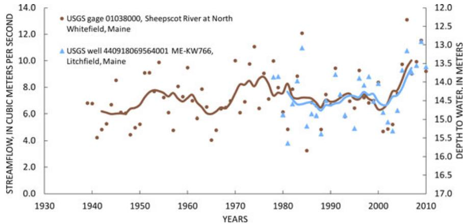
FIGURE 7. Graph Relating Month-End August Groundwater Levels with Annual Mean Streamflows. Streamflow record from a proximate (29 km) streamflow station is used to infer historical month-end August groundwater levels for periods of unavailable groundwater data. Curves are seven-year moving averages.
