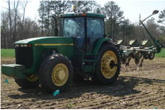
Fig. 1. John Deere 8300 MFWD with integral mounted KMC Generation I Rip-Strip unit used during this study.
