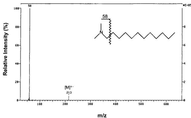
Figure 4. Electron ionization mass spectrum of the GC peak corresponding to *N,N*-dimethyl-1-dodecanamine. The mass spectrum is from an analysis of three handled glass beads.
