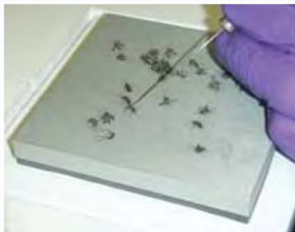
Figure 2: A repeating dispenser used for applying minute amounts of candidate insecticides to the thorax of adult mosquitoes. Mosquitoes are immobilized on a chill table.
