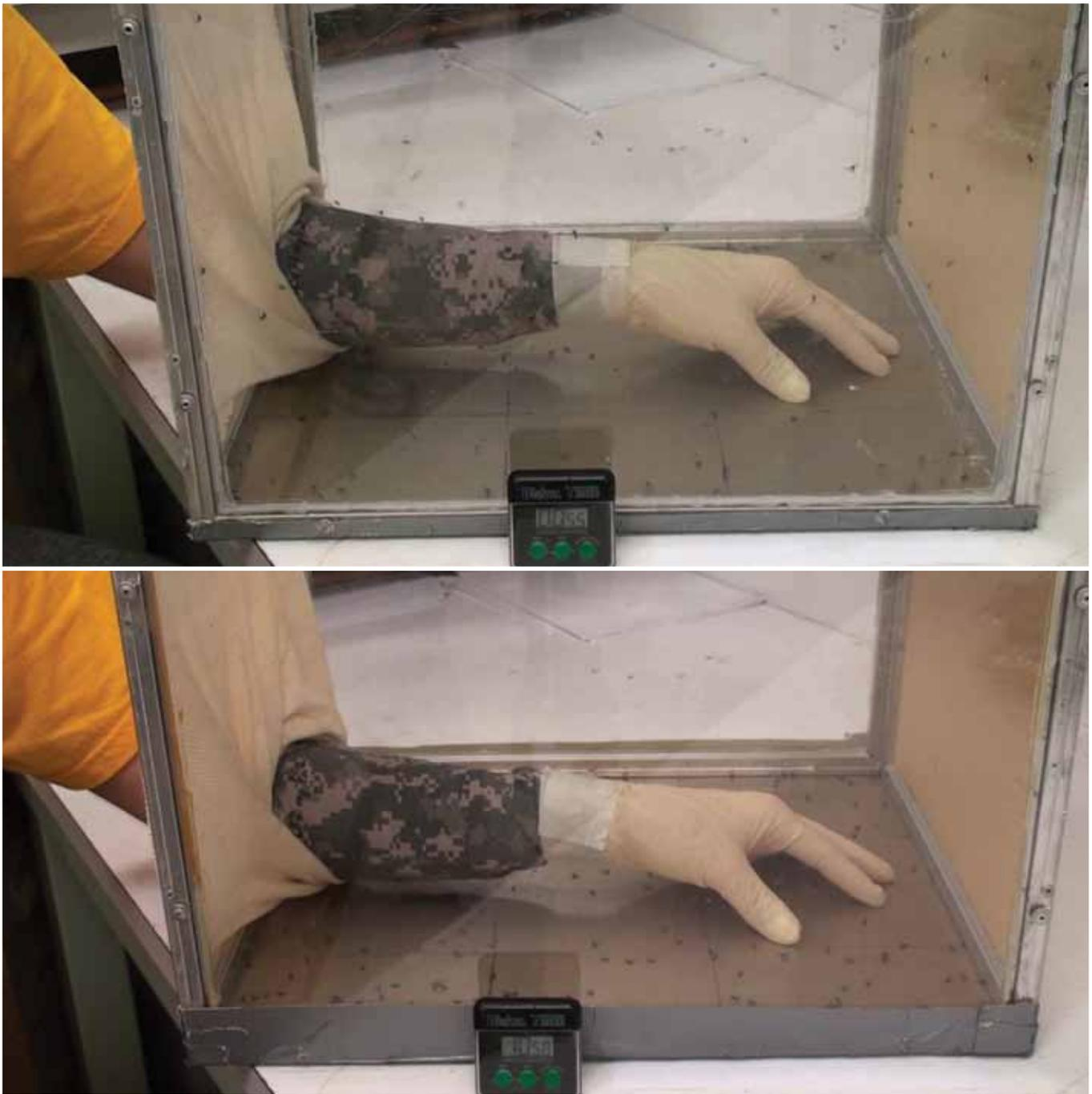
Figure 5: Comparison of mosquitoes surviving after 14 minute exposure to a permethrin Fire-Resistant Army Combat Uniform (FRACU) sleeve (top) and after 4 minute exposure to a FRACU sleeve treated with a fast-acting insecticide.
