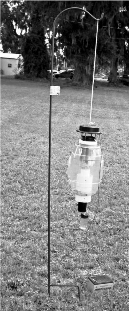
Fig. 1. Mosquito Magnet™-Experimental trap with jar of blend suspended near the carbon dioxide outlet port.
