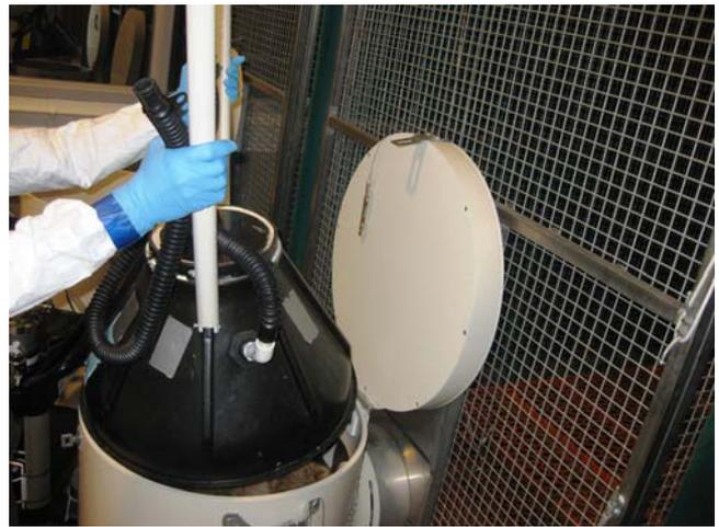
**Figure 1.** Cone-shaped anesthesia induction chamber measuring 36 cm high × 50 cm in diameter, with hinged manipulation handles, clear polycarbonate view port, and 22-mm vapor ports being inserted into a raccoon den chamber via a momentarily opened top hatch. The cone is designed to restrain an animal within the den chamber.
