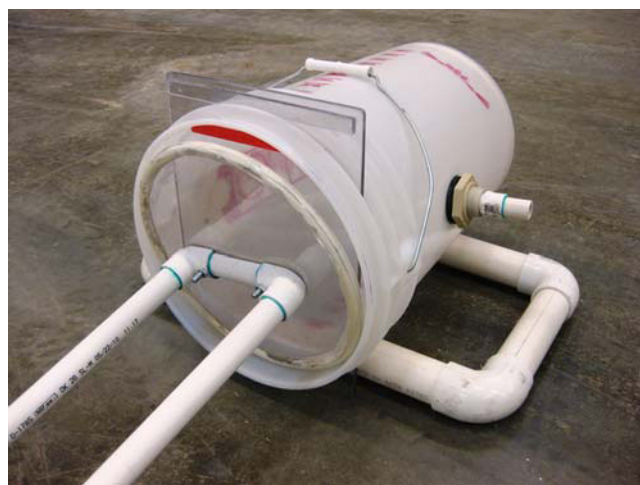
Figure 5. Cylinder anesthesia induction chamber with sliding door in place and plunger ready. Anesthesia hose attaches to the side-mounted vapor port shown.
