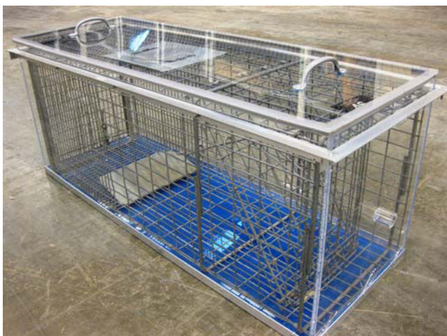
Figure 3. Box 1 anesthesia induction chamber with 81 cm × 25 cm × 30 cm live-catch trap and lid in place. A vapor port is visible on the right.
