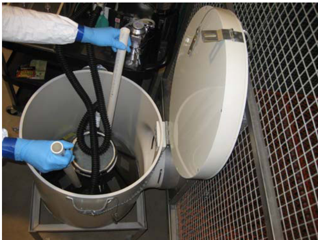
Figure 2. Den chamber with cone induction chamber fully inserted creating a final volume of 24 L. Isoflurane vapor is delivered via hoses attached to an anesthesia machine.
