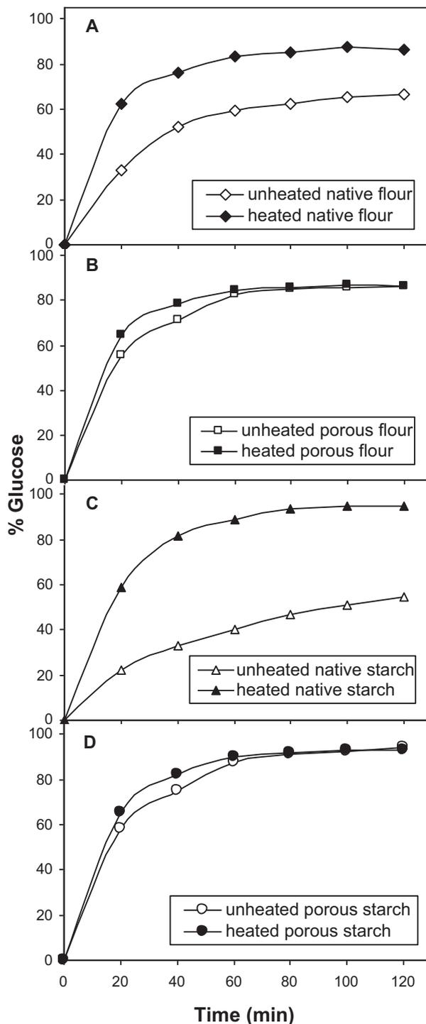
**Figure 4.** In vitro starch digestibility of unheated and heated native rice flour (A); unheated and heated pregelatinized rice flour (B); unheated and heated native rice starch (C); and unheated and heated pregelatinized rice starch (D).
