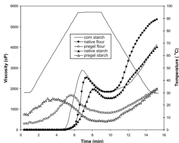
**Figure 2.** Rapid visco analyzer (RVA) pasting profiles of native and pregelatinized (pregel) rice flour and starch samples in comparison with a corn starch standard.
