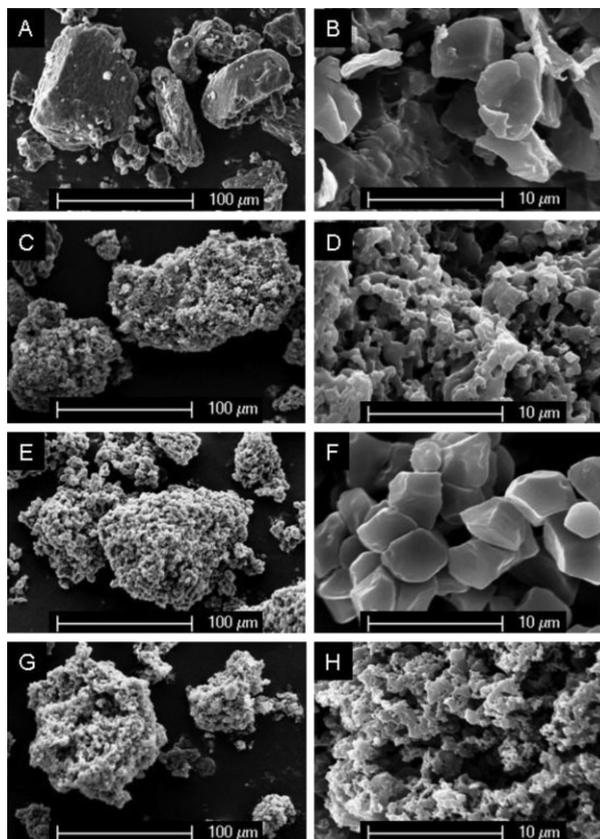
**Figure 1.** Low ( $1000\times$ ) and high ( $2500\times$ ) magnification scanning electron micrographs, respectively, for native rice flour (A and B), porous rice flour (C and D), native rice starch (E and F), and porous rice starch powder (G and H).
