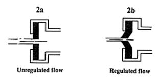
Flow Control Nozzle nearly constant flow rate out of a sprinkler.
