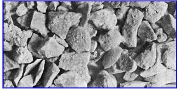
**Figure 1. Ag lime separated by sieving into the three size ranges.**
