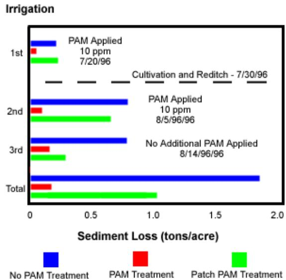
Figure 2. Sediment loss (tons/acre) for each irrigation and total sediment loss (tons/acre) for treatments of no PAM, PAM and patch PAM (1996).
