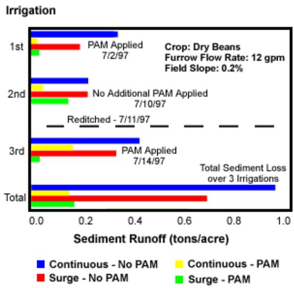
Figure 4. Sediment loss (tons/acre) for each irrigation and total sediment loss (tons/acre) for treatments of no PAM – continuous irrigation, PAM – continuous irrigation, no PAM – surge irrigation and PAM – surge irrigation (1997).
