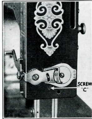
Courtesy of White Sewing Machine Co. FIG. 9.—Screw "C" also adjusts needle centering.
