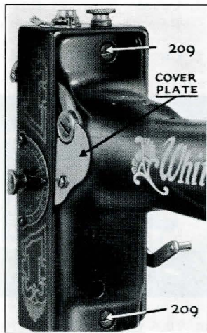
Courtesy of White Sewing Machine Co. FIG. 8.—Loosen these screws to adjust needle centering or take-off end housing.
