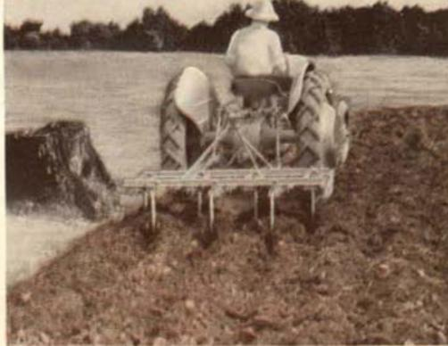
Tilling 5 feet wide and 10 inches deep with new-type tillage tool. Ideal for orchard cultivation and tillage work.
