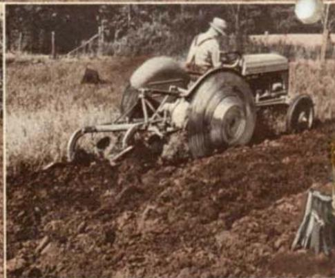
*Obstructions?* Demonstration proves that Ford tractor with Ferguson system "line of draft" is its own safety device.
