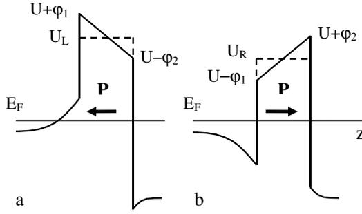
FIG. 2. Schematic representation of the potential profile  $V(z)$  in a  $M_1$ -FE- $M_2$  junction for polarization pointing to the left (a) and for polarization pointing to the right (b), assuming that  $\delta_1 > \delta_2$ . The dashed lines show the average potential seen by transport electrons tunneling across the ferroelectric barrier. The horizontal solid line denotes the Fermi energy,  $E_F$ .
