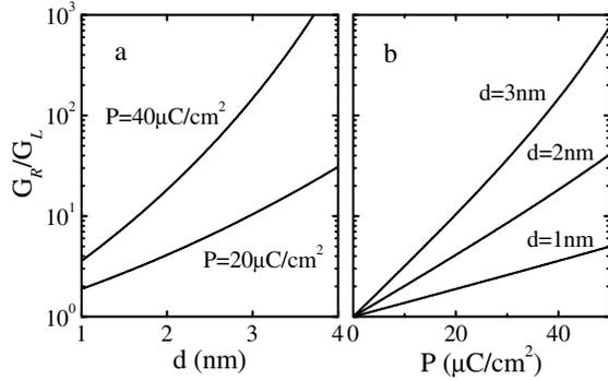
FIG. 4. GER ratio,  $G_R/G_L$ , as a function of ferroelectric barrier thickness  $d$  for different values of polarization (a) and as a function of polarization  $P$  for different barrier thicknesses (b).  $\delta_1 = 6 \text{ \AA}$ .
