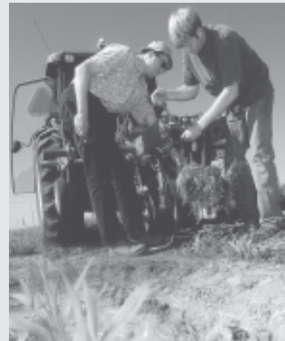
Biological Systems Engineer Viacheslav Adamchuk (left) and graduate student Philip Christenson adjust the alignment of sensors during a field test of new soil sensors. Adamchuk is developing these sensors to help farmers better understand and manage differences in their soil across fields.
