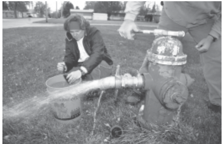
IANR water scientists are working with small towns on lower cost ways to reduce arsenic levels in public water supplies. Here, Lynn Klawer, project coordinator, collects a sample from a small community's water main.
