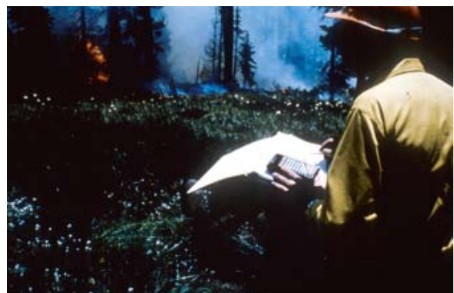
Dick Rothermel uses a TI-59 calculator programmed with his fire spread model on a fire site circa 1983.
