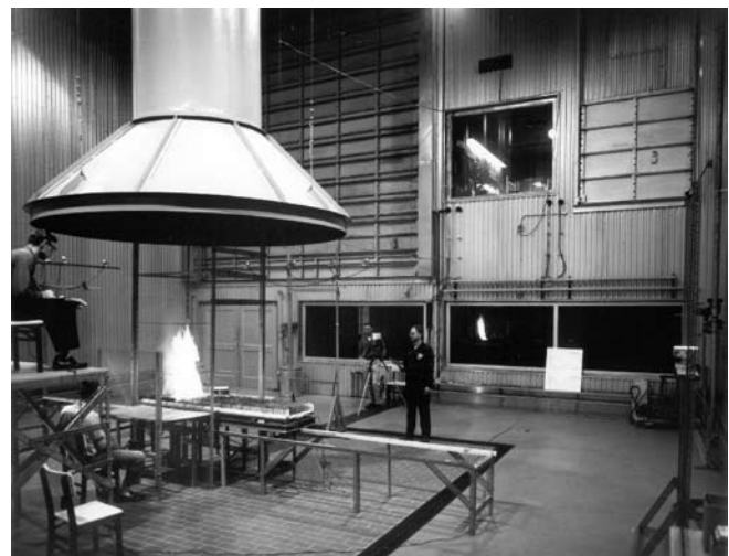
Combustion chamber at Missoula Fire Lab; photo taken in the mid-1960s.
