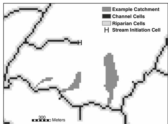
**Fig. 3** Examples of riparian catchments, channel cells, and riparian cells using 30-m cells in part of Keg and Silver Creek basins (Burkart et al. 2004). The ‘example catchments’ indicate the contributing area ( $A_s$ ) for three selected riparian grid cells
