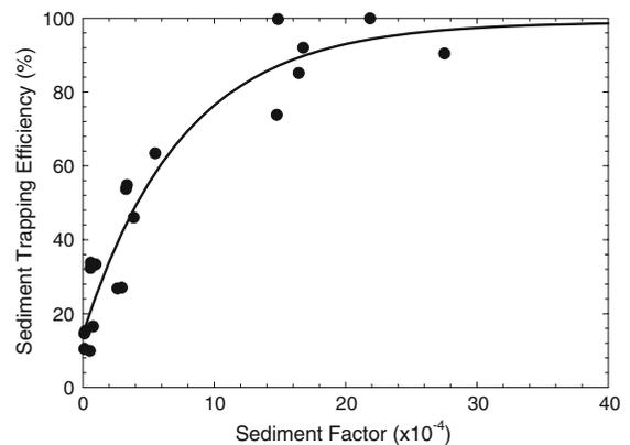
**Fig. 1** Comparison of sediment factor values and corresponding values for sediment trapping efficiency (percent of input load deposited in the buffer) (Dosskey et al. 2006) estimated using VFSSMOD (Muñoz-Carpena and Parsons 2000). The fitted curve is given by Eq. 2
