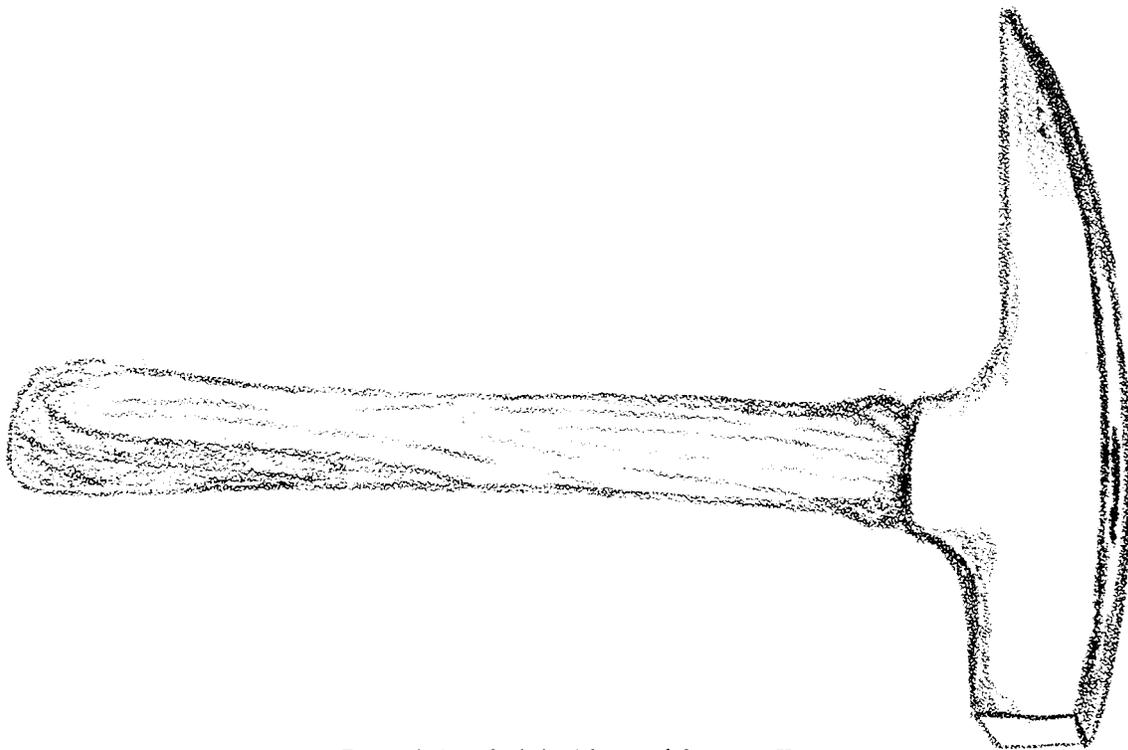
FIGURE 4. A geologist's pick or rock hammer, X $\frac{1}{2}$ .
