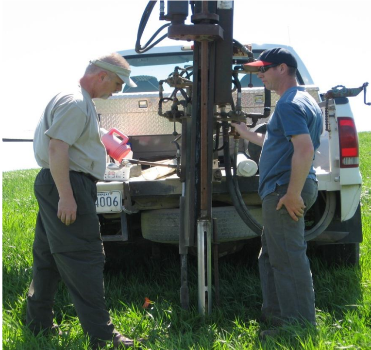
Figure 3.2 Core collection. Cores from the stream banks near the knickpoint face were collected using a Giddings probe and Shelby tube system (cont'd. next page).
