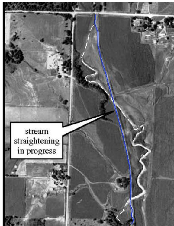
Figure 1.1 (a) Channel straightening of Mud Creek, IA in the 1950s. The white line is the original channel. The blue line is the creek after straightening.
