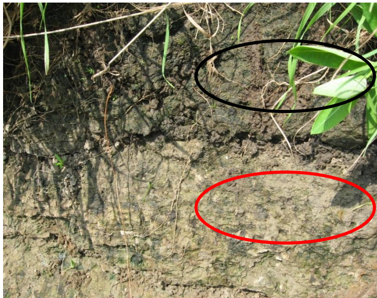
Figure 4.1 Stratigraphic discontinuity. There appears to be a stratigraphic discontinuity close to the knickpoint with a darker sediment (in the black circle) overlaying a lighter-colored sediment (in the red circle).
