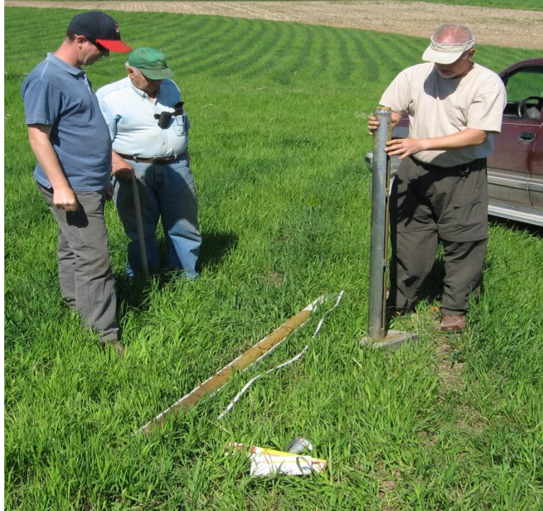
Figure 3.2 (cont'd.) Core collection. Cores from the stream banks near the knickpoint face were collected using a Giddings probe and Shelby tube system
