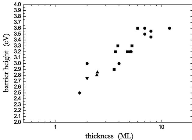
FIG. 8. Measured barrier height vs thickness of MgO for slightly different positive-bias voltages. The symbols correspond to the following biases:  $\square$  (+4.09 V),  $\circ$  (+4.01 V),  $\triangle$  (+3.55 V),  $\nabla$  (+3.21 V), and  $\diamond$  (+3.08 V).
