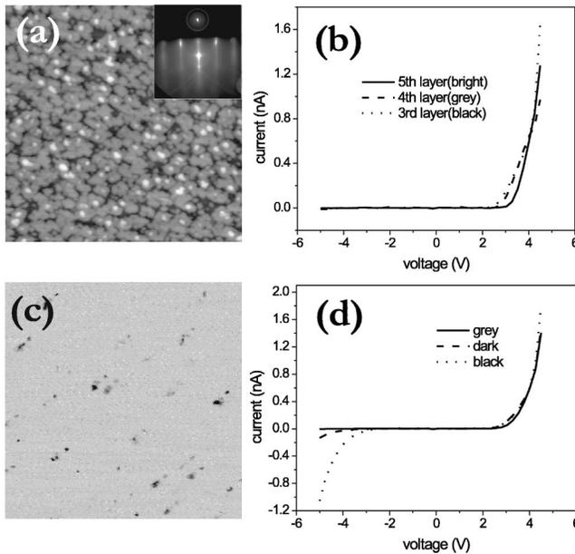
FIG. 5. (a) Morphology of 3.8 ML MgO on Fe(001), rms roughness: 0.075 nm (+4.1 V, 0.66 nA,  $100 \times 100$  nm<sup>2</sup>). The inset shows a RHEED pattern along a [110] crystallographic direction of MgO. (b) Tunneling spectra for different thicknesses of MgO shown in (a). (c) Spectroscopic current image of local defects taken at a bias voltage of  $-4$  V ( $100 \times 100$  nm<sup>2</sup>). (d) Tunneling spectra of a defect free area (gray) and of different local defects (dark and black).
