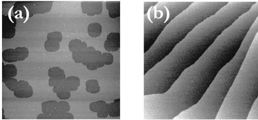
FIG. 1. STM topographical images: (a) Clean Fe(001) whisker (tunneling conditions: +0.6 V, 0.6 nA,  $2000 \times 2000 \text{ nm}^2$ ). (b) Clean Fe(001) bulk crystal (tunneling conditions: +0.54 V, 0.66 nA,  $500 \times 500 \text{ nm}^2$ ).
