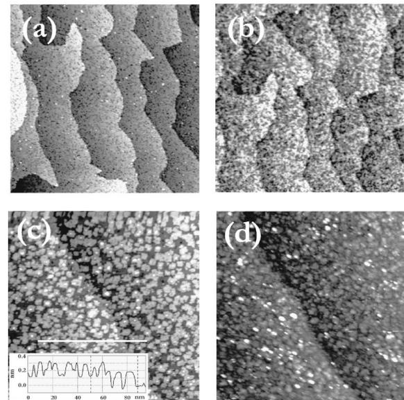
FIG. 4. STM topographic imaging of MgO layers on Fe(001) in dependence on bias voltages. (a) 1.9 ML MgO, rms roughness: 0.063 nm (+3 V, 0.66 nA,  $300 \times 300$  nm<sup>2</sup>). (b) 1.9 ML MgO (+4 V, 0.66 nA,  $300 \times 300$  nm<sup>2</sup>). (c) 3.6 ML MgO, rms roughness: 0.074 nm (+4 V, 0.8 nA,  $150 \times 150$  nm<sup>2</sup>). Inset shows plot of topographical height vs position along a horizontal line. (d) 3.6 ML MgO (+2 V, 0.3 nA,  $150 \times 150$  nm<sup>2</sup>).
