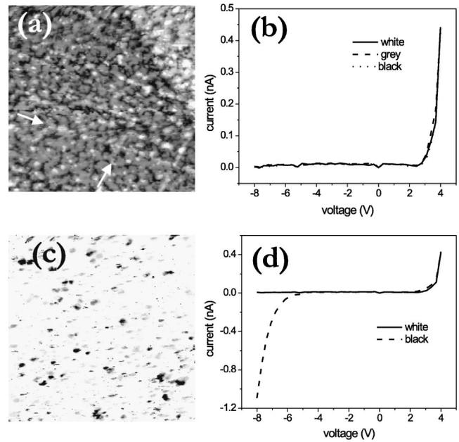
FIG. 7. (a) Morphology of 7 ML MgO on Fe(001) exhibiting dislocation traces (arrows), rms roughness: 0.092 nm ( $+4$  V, 0.29 nA,  $100 \times 100$  nm<sup>2</sup>). (b) Tunneling spectra for different thicknesses of MgO shown in (a). (c) Spectroscopic current image of local defects at a bias of 8 V ( $100 \times 100$  nm<sup>2</sup>). (d) Tunneling spectra from defect free areas (solid) and from local defects (dashed) shown in (c).
