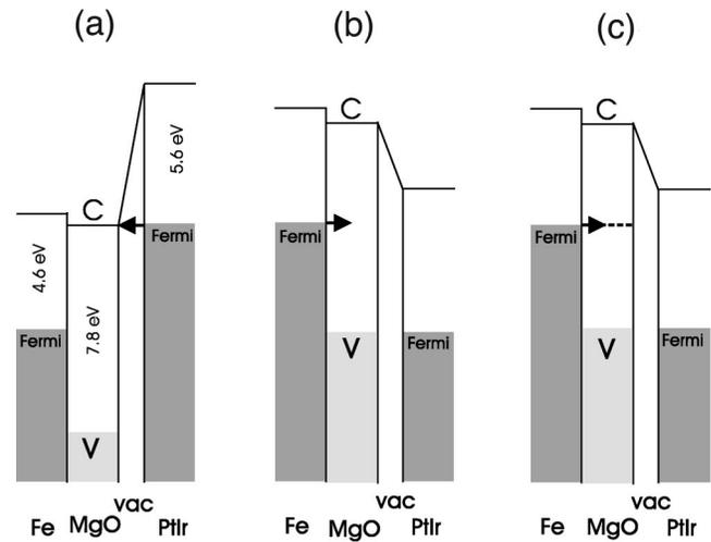
FIG. 6. A sketch of energy bands of the Fe/MgO/vacuum/PtIr tip structure. (a) Bias voltage  $+4$  V, tunneling into the conduction band of MgO through the vacuum barrier. (b) Bias voltage  $-4$  V, tunneling from the valence band of MgO through the vacuum barrier. (c) Negative-bias voltage, tunneling through additional defect states midway between the valence and conduction bands of MgO.
