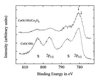
FIG. 4. XP core region for CoO(100) and the Co<sub>3</sub>O<sub>4</sub> epitaxy taken with Mg  $K_{\alpha}$  radiation and a band pass of 50 eV. The arrows in the spectrum for CoO(100)/Co<sub>3</sub>O<sub>4</sub> epitaxy indicate core emission associated primarily with Co<sup>3+</sup> (779.6 eV) and Co<sup>2+</sup> (780.5 eV) cations in the spinel structure.
