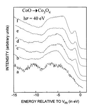
FIG. 2. Valence-band spectra at 40 eV for the CoO(100) substrate heated at 623 K and  $1 \times 10^{-4}$  Torr O<sub>2</sub> for (a) 0 h, (b) 0.5 h, (c) 1.0 h, (d) 2.0 h, (e) 3.0 h, and (f) 4.0 h. The latter spectrum corresponds to epitaxial Co<sub>3</sub>O<sub>4</sub>.
