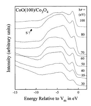
FIG. 6. Photoemission from the  $Co_3O_4$  epitaxy taken at normal emission and as a function of primary beam energy. The feature indicated by *S*? is potentially associated with  $3d^{n-1}$  final state.
