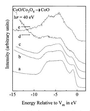
FIG. 7. Photoemission from the valence-band region of the  $CoO(100)/Co_3O_4$  surface as it is heated to progressively higher temperatures: (a) no heating, (b) 773 K, (c) 873 K, (d) 973 K and (e) 1073 K. Spectra were acquired at normal emission and 40 eV primary photon beam.
